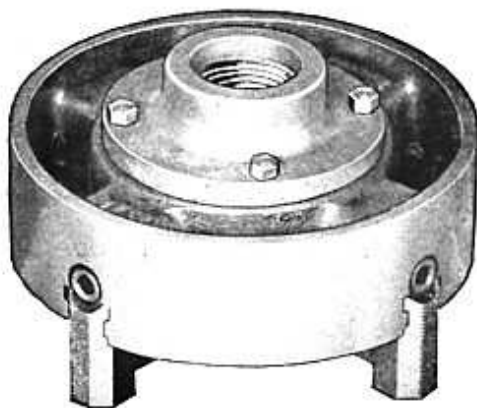
Fig. 506.—Chuck with Chuck Plate attached
