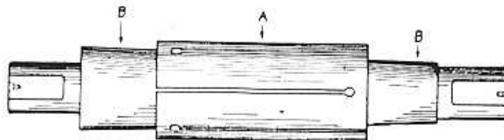
Fig. 480.—An Expanding Mandrel
