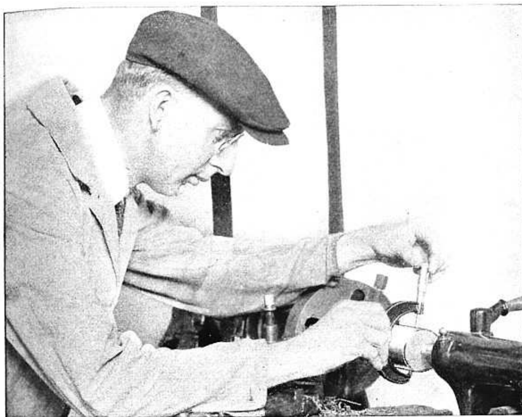
Fig. 439.—Using a Micrometer Caliper Measuring Work in the Lathe
